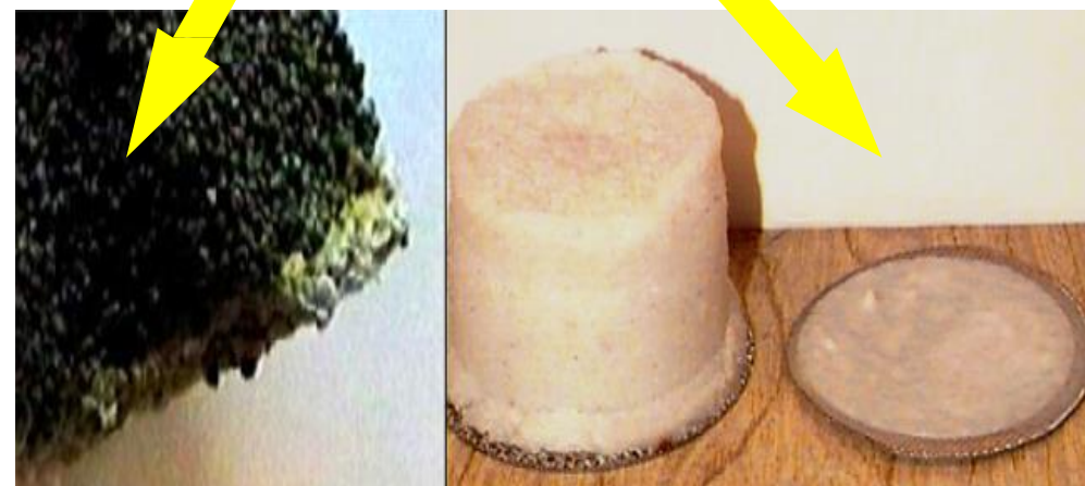
Filter cakes: optimal (right) and nonoptimal (left)
